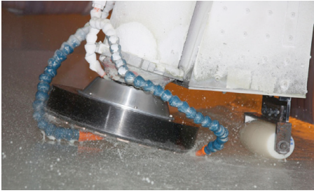
Grinding wheel removing glass from the LSST tertiary mirror.
