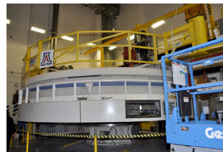
LSST mirror blank on the Large Optical Generator
