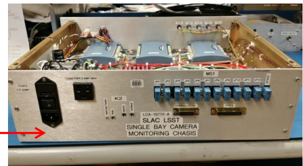
Single Bay Camera DAQ Module
