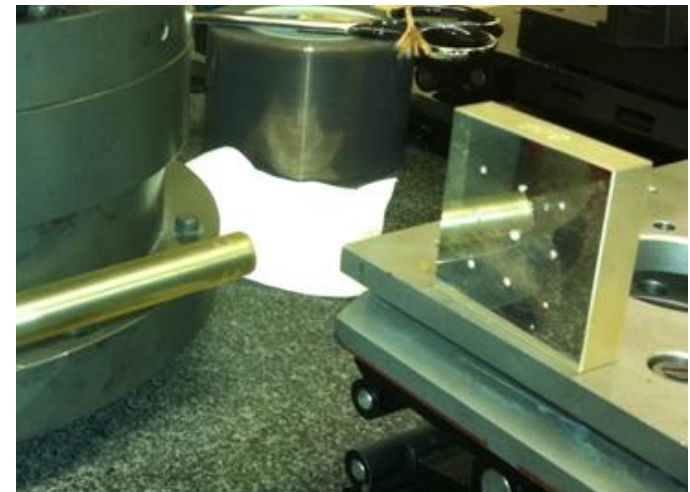
Small coated Borosilicate sample with holes under test
