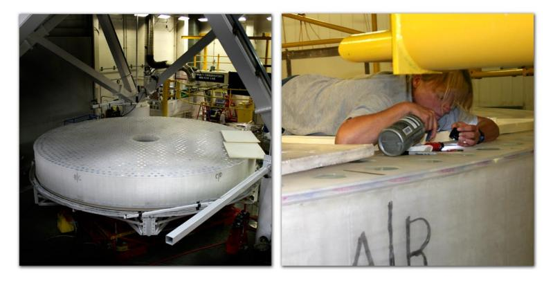
The Steward Observatory Mirror Laboratory has completed the rough abrasive grinding of the 8.4-meter LSST M1/M3 mirror back surface (left). Technician Leslie Utley (right) carefully inspects the back surface of the monolithic mirror blank for imperfections. The back surface will undergo polishing over the next several weeks. Support hardware will then be bonded to the back surface and the mirror carefully turned so optical polishing of the front surface can begin later this year.
