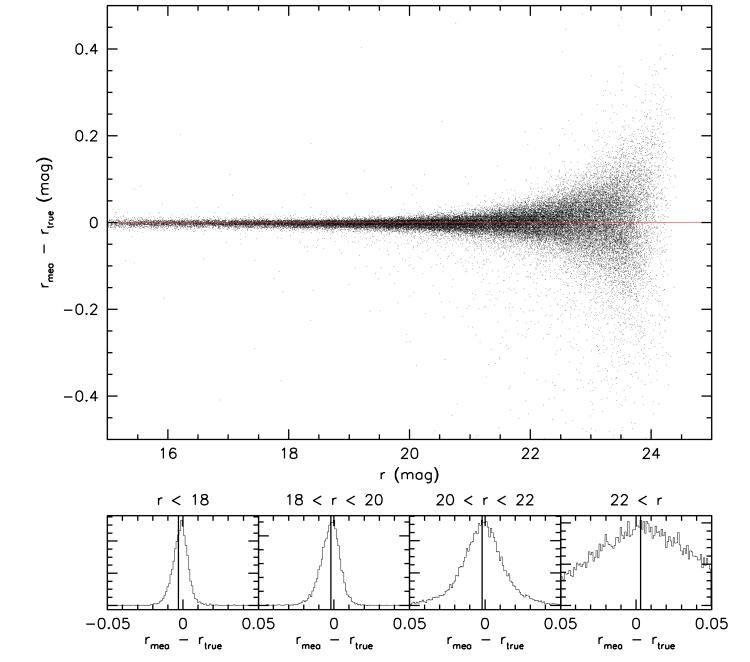
**Above:** The accuracy of LSST photometry. We have crossmatched the objects detected in simulated visits to the input ("truth") catalogs, and compared measured vs. true magnitudes for point sources. The current DM pipeline produces 2 mmag of bias and about 7 mmag RMS scatter at bright magnitudes. While not yet at the required levels, this is sufficient to test the capability to detect and characterize ultra-faint dwarf galaxies.
