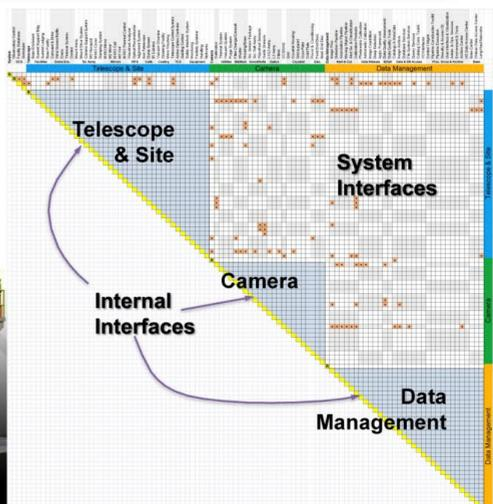
Interfaces define the interactions of the system components. There are 98 x 98 possible intersections between the LSST's three subsystems and their major components.
