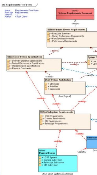
**Requirements Hierarchy:** The requirements flow down in LSST generally follows the hierarchy shown in the diagram (below-left). The operational requirements are derived from the Operations Models (left). The Functional Requirements flow directly from the SRD or are derived from a variety of sources including the Operations Simulator, Exposure Time Calculator, site characteristics, optical design, etc.
