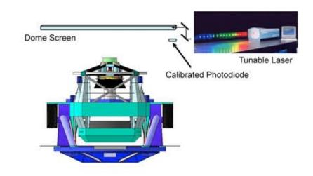
A photodiode calibrated to  $\sim 0.1\%$  relative accuracy (NIST98) from 450nm to 950nm monitors the integrated optical exposure. Spatial uniformity of light from the screen need only be  $\sim 10\%$ , but the angular distribution must be uniform (Lambertian) over the 3.5° LSST FOV. First tests of a similar system on the CTIO Blanco telescope have been reported (Stubbs 2007b).
