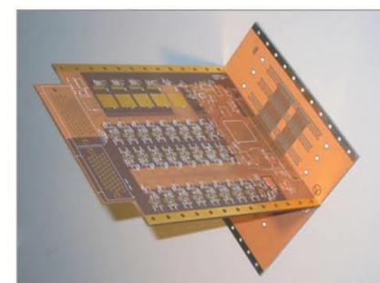
8 Channel Prototype ASIC Test PCB
