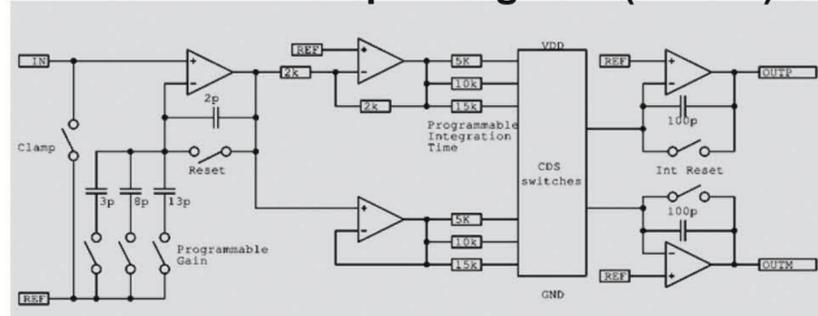
Prototype CCD Readout ASIC V1
