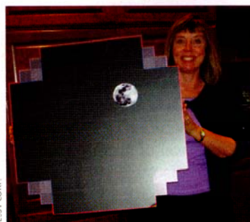
BIG PICTURE The heart of the LSST will be a 3,200-mega-pixel CCD array. On this mockup, the full Moon (about \frac{1}{2}^\circ wide) illustrates the image scale on the sky. Image sensors in the corners will handle guiding and tracking.
