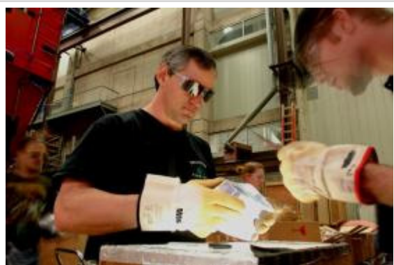
Casting team supervisor Randy Lutz and team inspected 52,900 pounds of glass for the LSST primary/tertiary mirror. A total 51,900 pounds of glass will be loaded into the mold. (Ray Bertram, Steward Observatory)
