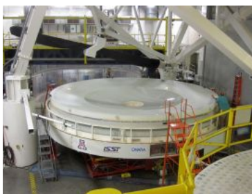
The unique primary mirror with the integrated tertiary mirror in its center will form the heart of LSST. (Photo by SOML/LSST Corp.)
