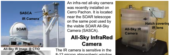
All-Sky InfraRed Camera The IR camera is sensitive in the 8-12 micron atmospheric window. It includes six filters, one wide-band filter and five narrow-band filters. The system uses an IR fish-eye lens to get a 180deg field of view. A black body located in the protective lens hatch cover is used periodically during the night to get a reference image. During regular night operation, the LSST scheduler will be used to select fields.
